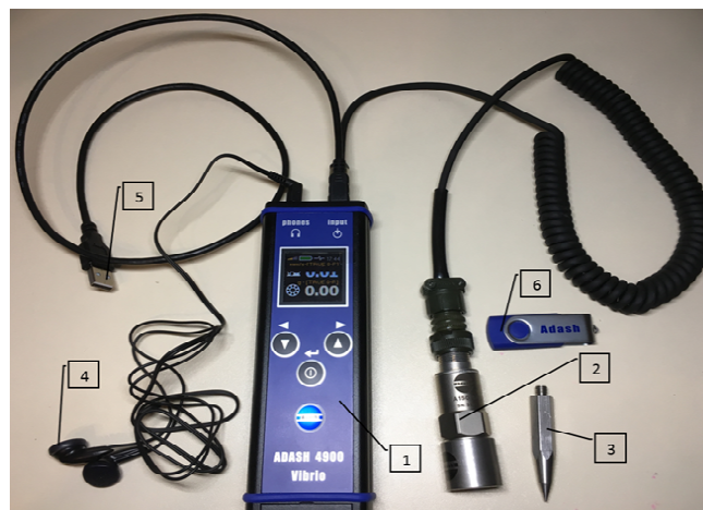
Fig. 1. Vibration analyser A4900 Vibrio M from „Adash” company: 1 – analyser and data collector; 2 – accelerometer with magnetic base; 3 – measuring tip for manual pressure on the sensor; 4 – headphone set; 5 – USB connection; 6 – USB stick
